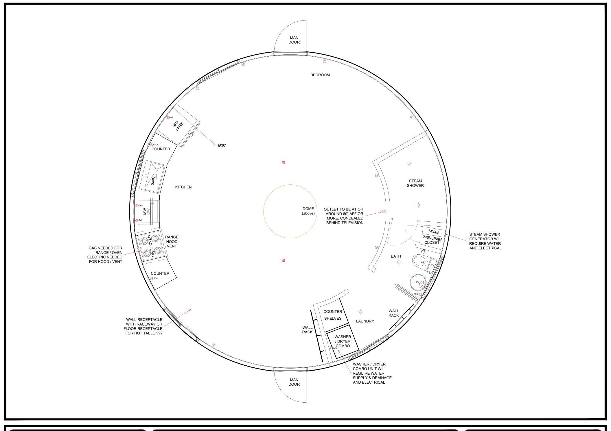
30' YURT FLOOR PLAN Proposed Gas/Electrical - Model A
