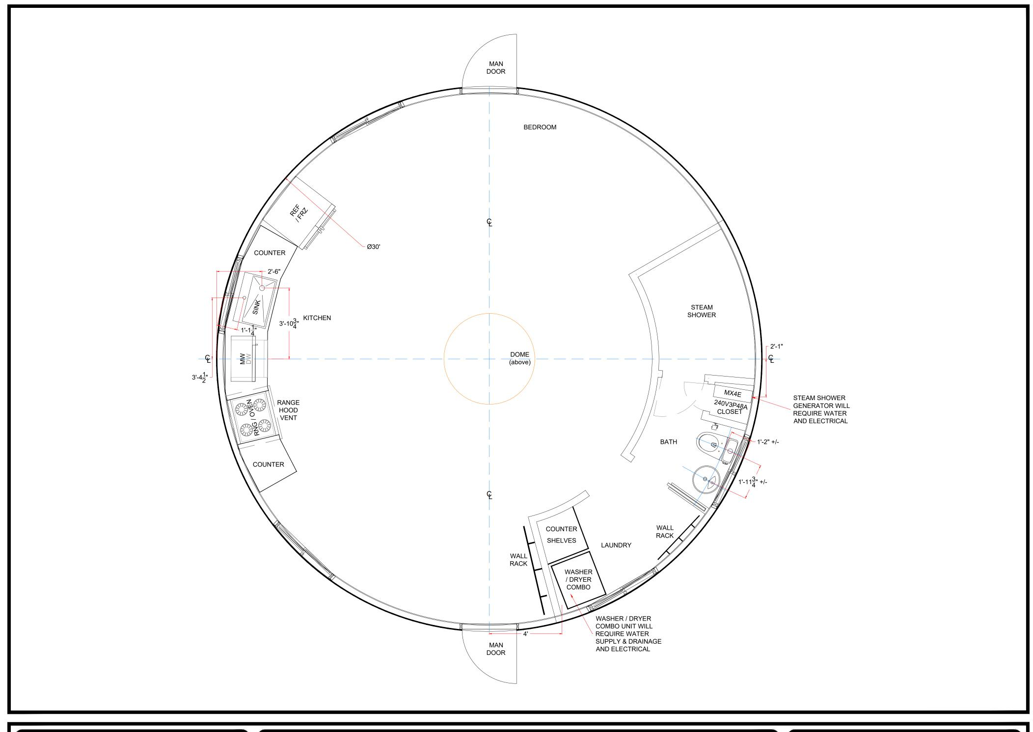
30' YURT FLOOR PLAN Proposed Water Plan - Model A
